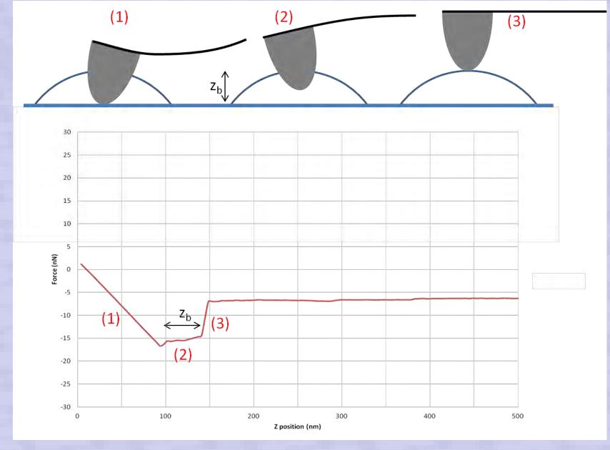
Plateaus observed in the retraction curve correspond to the maximum extension of the bubble when attached to the tip.
