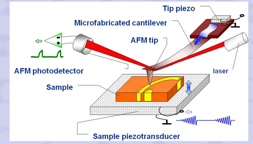
Ultrasonic (UFM) force microscopy combines the nanoscale resolution of the AFM with the elastic sensitivity of acoustic microscopy. ultrasonic High frequency vibrations are applied to the sample forcing it to elastically indent itself against an AFM tip which is very stiff at MHz frequencies.
