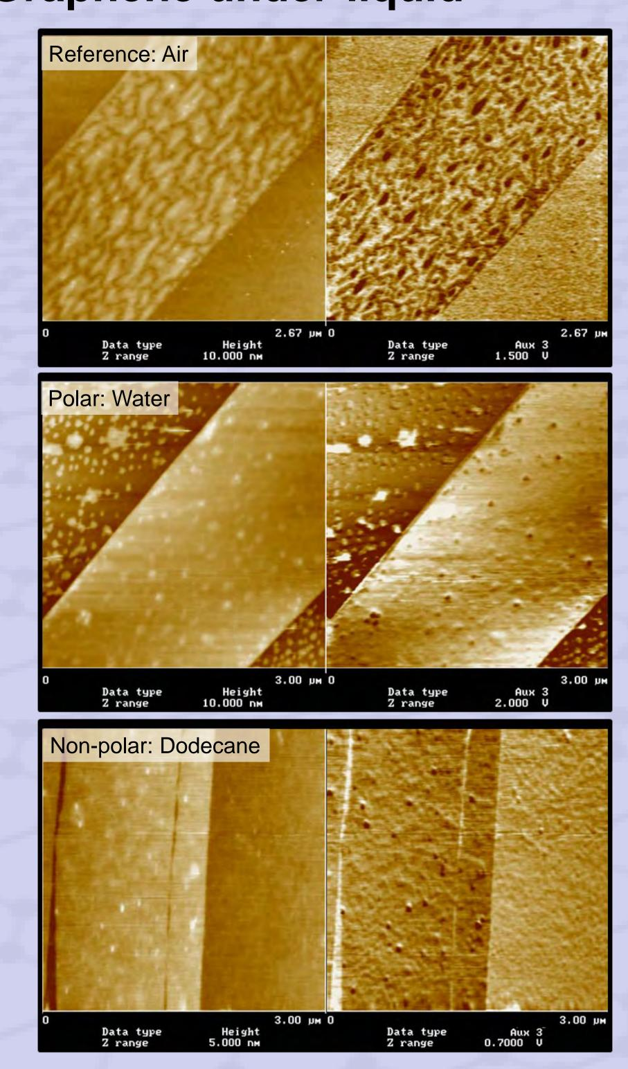
An exfoliated graphene flake on a SiO<sub>2</sub> substrate was imaged using both contact AFM and UFM in air (top), water (middle) and dodecane (bottom) environments. Thus topography, friction and elastic response can be mapped for the same region.
