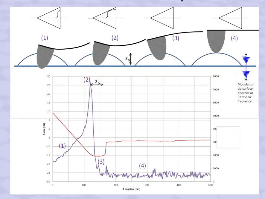
UFM response shows a detachment from the solid-solid contact prior to snap out of the tip, suggesting that forces experienced by the tip in the plateau region are not directly due to the graphene flake.
