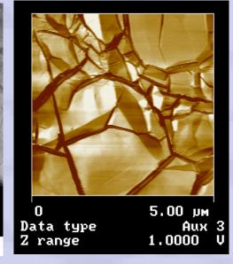
Also, a 6mm diameter Ir(111) single crystal homogeneously covered with single layer graphene of high structural quality.
